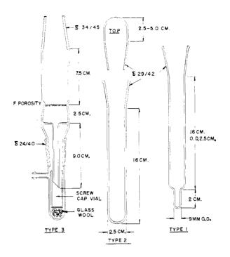
Figure 1. Special apparatus used in the procedure
